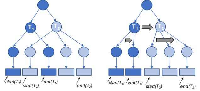
Figure 1: Task interleaving (left) vs. totally ordered (right).
