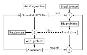
Figure 1: Protocol description. Rectangles represent information or data structures managed by the agents. Blocks on the left are managed by the auctioneer, blocks on the right by each bidder. Dashed arrows represent data exchanged between the auctioneer and the bidders. Circles indicate processes that aggregate information to build new structures. Double arrows indicate calls to a HTN planner.
